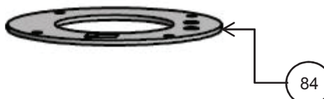
White Ceramic Gasket (only required if heat exchanger surface is rough or uneven)
